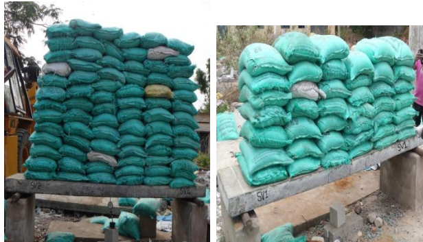
Fig 3 Live load with sand bags on test slabs.
